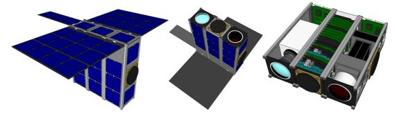
Figure 1 – Imager spacecraft configuration with Multi-Spectral Imager and microbolometer payload.
